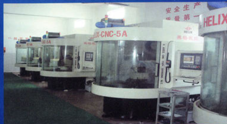
产品源自五轴联动数控工具磨床 Products derived from 5-axis CNC tool grinder
