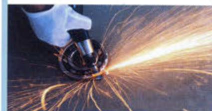
切削硬度HRC62的轴承钢图例 Cutting the hardness HRC62 bearing steel Legend
